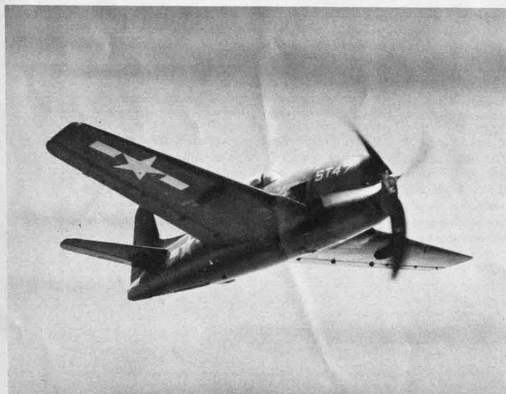
Belly line of the new Grumman fighter is practically straight. The area of its tall, angular fin and rudder has been increased by the addition of a dorsal fin for greater lateral stability.
